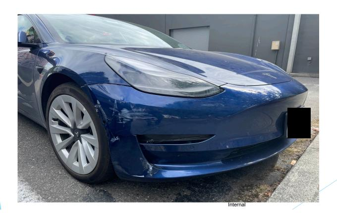
Bumper cover is broken, parking sensor is missing, splash shield is torn but is difficult to see in previous photo.
